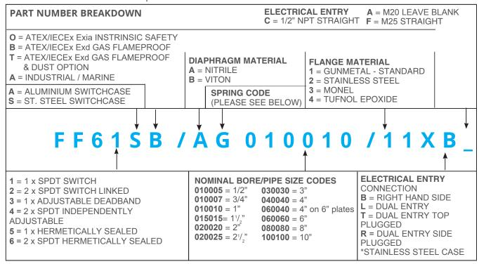
Spring code: This will be designated by our Engineer upon calculating the most applicable orifice ratio dependent on the pipe size, normal flow and alarm flow required for your specific application. These calculations will give a figure in "HG and the spring codes cover specific ranges.
